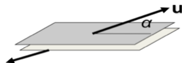
Figure. 1. The schematic model of tensile earthquake; the slip vector is deviated from fault plane by \alpha .
