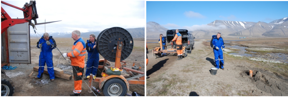
Figure 2: Left: Installation of the 5-level 3C-geophone string at the CO 2 lab. Right: deployment of borehole seismometers at 12 m depth, well within the permafrost.
