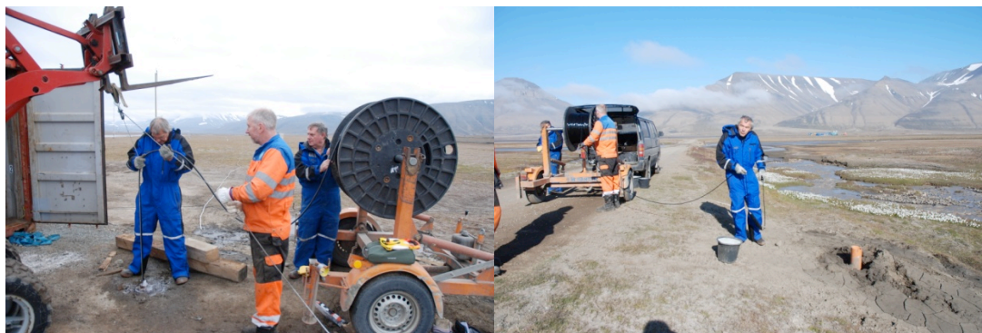
Figure 1: left: Installation of the 5-level 3C-geophone string at the CO 2 lab. Right: deployment of borehole seismometers at 12 m depth, well within the permafrost.
