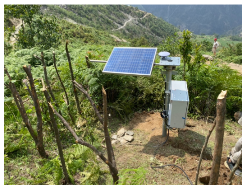
Figure 3: Seismic station deployed on the Bolde landslide, central Nepal, showing the broadband sensor, solar power system, and GNSS antenna.
